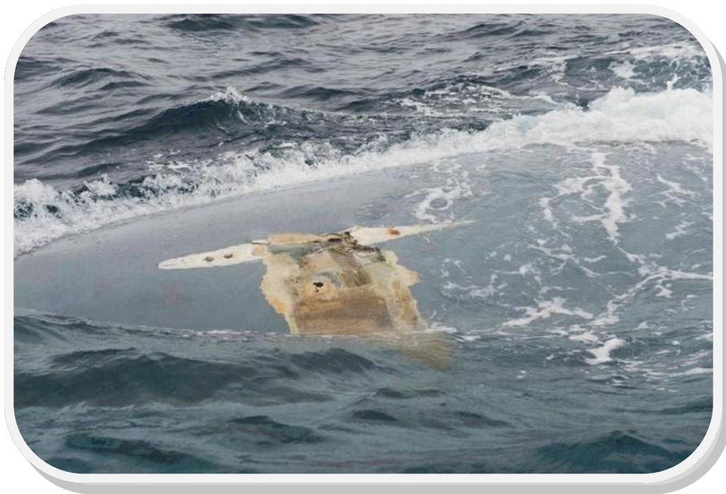
The keel is gone, and the laminate has been torn away leaving large holes
