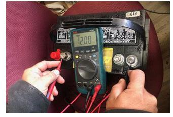
Test the for voltage by placing the red lead on the positive wire (brown), and the black lead on the negative wire (black). You should read battery voltage. If no voltage is shown, check the wiring, fuses and breakers between the battery and the bilge pump. If voltage is seen, but the pump doesn't operate, check for a blockage in the pump, or evidence of overheating/melting. Repair/replace as necessary.
